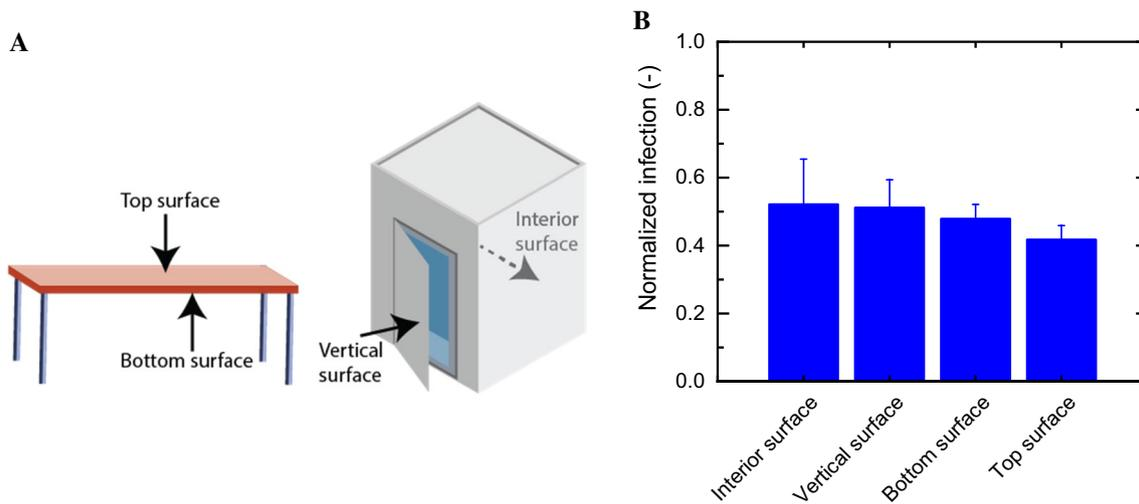
**Fig. 4** **A** Positions by which a contaminated glass surface was placed and ozonated. **B** Ozone disinfection of several surface positions. Surfaces were contaminated with SARS-CoV-2-Spike pseudoviruses
